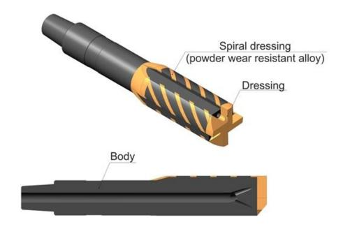
The Special Junk Mill consists of body made of high-strength alloy steel and cutting and grinding dressing with crushed tungsten carbide introduced into matrix of nickel-containing brass. Blades are dressed with powder alloy "Eutalloy" in order to reduce wear and tear of body.
